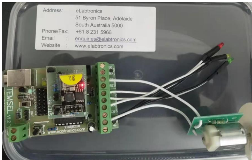
Figure 7 Circuit connection on STEMSEL.
